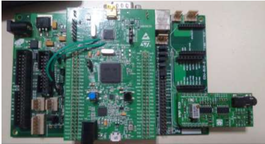
Fig.3.1 The ECG sensor is connected to the CORTEX M4 bit
