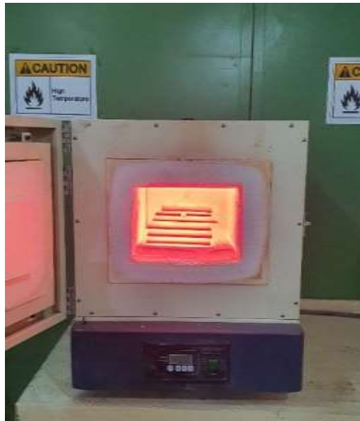
Figure (4) Coupons and specimens heated in a Furnace
