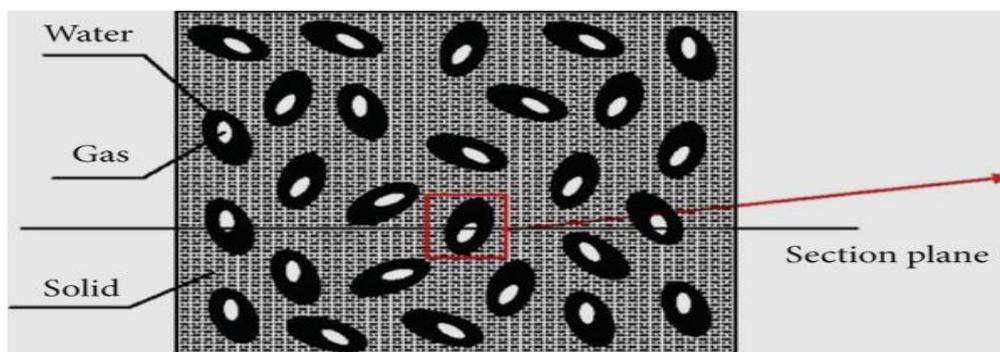
**Fig.4: Fractal Model to Interpret Porosity-Dependent Hydraulic Properties for Unsaturated Soils.**
