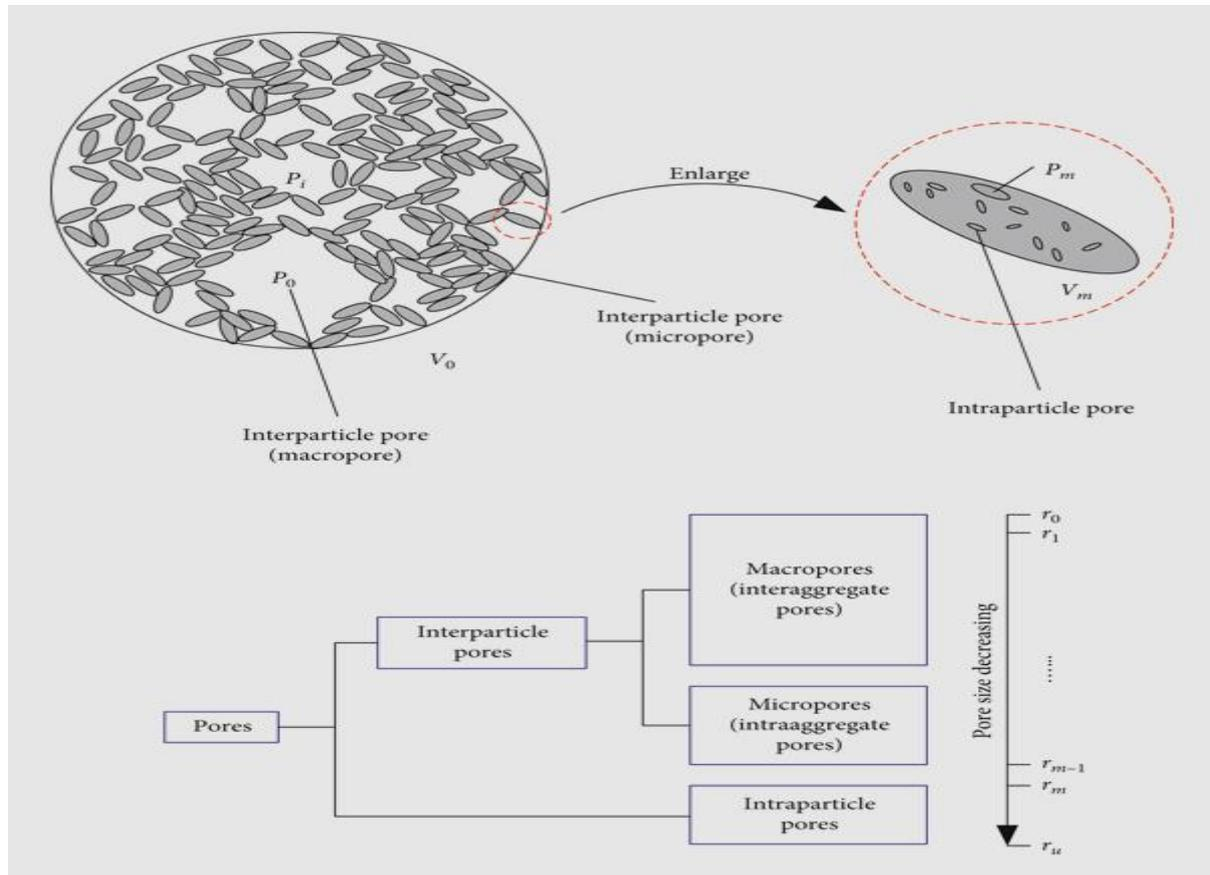
Figure 1: Characterization of pores.
