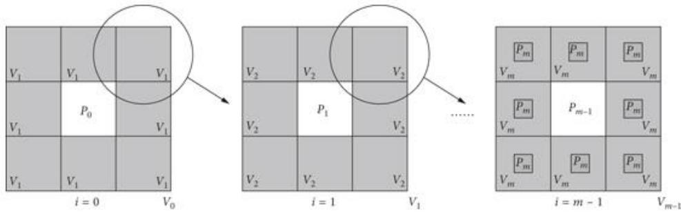
Figure 2: Schematic diagram of fractal porous medium (Sierpinski carpet).
