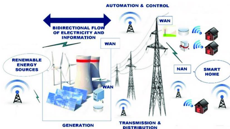
Figure 1. Smart grid communication infrastructure [10].
